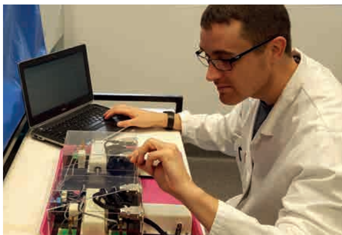
Dr David Musson operates the ‘Cell Gym’, a device used for the application of mechanical strain on bone and muscle cells.
